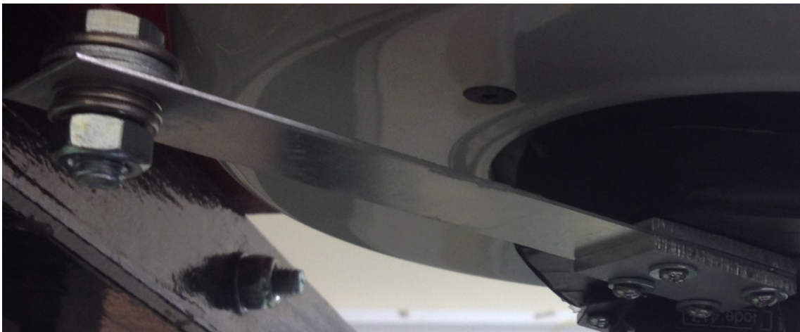
Figure 2: Cantilever Device for Energy Harvesting from Train Induced Vibrations in Bridges. Source: Author
